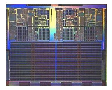
The top left and right hand side of the CPU contain the actual processing cores that do the calculation. The darker areas under each core contain the cache (a form of super-fast RAM).
