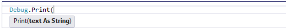
Figure 68: Parameter Info box showing that the Print method expects a single string parameter.
