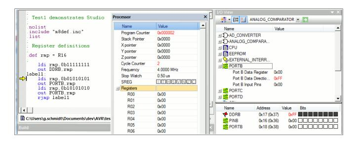
The instruction "Out DDRB,rmp" writes 0xFF to a port named DDRB. Now the action is on the I/O view window. If you push on PORTB and the small "+" left of it, this window displays the value 0xFF in the port DDRB in two different forms: as 0xFF in the upper window portion and as 8 black squares in the lower window section.
