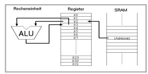
Unit ALU, sometimes called accumulator) like the registers are. If you access these memory locations you usually use a register as interim storage. ln the example displayed here a value in SRAM will be copied to the register R2 (1st instruction), a calculation with the value in R3 is made and the result is written R3 (second to instruction). After that this value is written back to the same SRAM location (instruction 3, not shown here).
