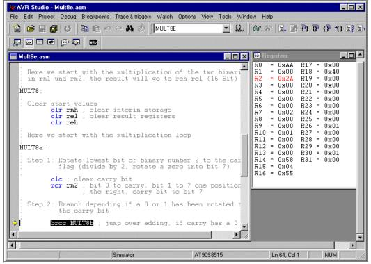
Because the carry bit had a one, the content of the registers R1:R0 is added to the (empty) register pair R4:R3, resulting in 0x00AA there.
