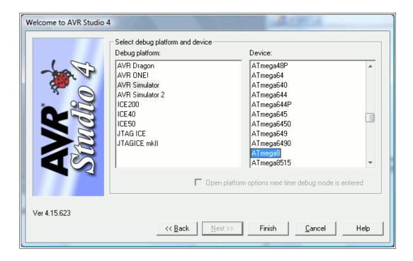
As debug platform select either "AVR simulator" or "AVR simulator 2". As Device select your AVR type, here an ATmega8 was selected. If your desired type is grayed out, select another simulator platform. Close this window with the "Finish" button. Now a large window pops up, which has lots of different subwindows.
