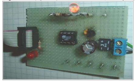
The hardware can be build on a small board like the one shown in the picture. All pins of the tiny13 are accessible, and external hardware components, like the LED shown, can be easily plugged in.
