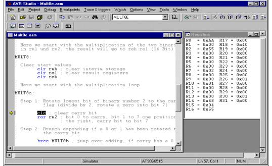
R2 is rotated to the right, to roll the least significant bit into the carry bit. 0x55 (0101.0101) yielded 0x2A (0010.1010).
