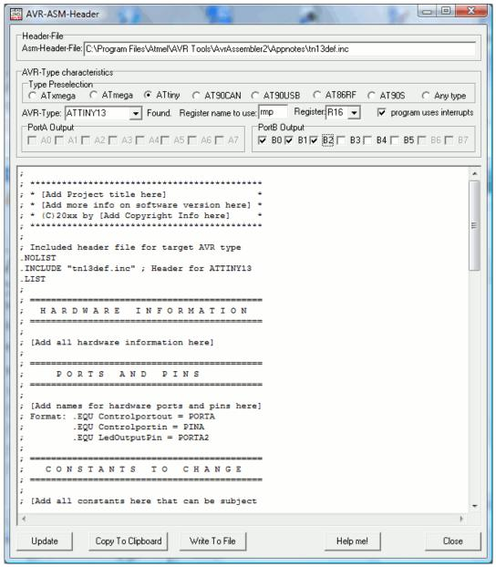
Here you can enter your desired multi purpose register, the output configuration on ports A and B, if available, and if you want to use interrupts.
