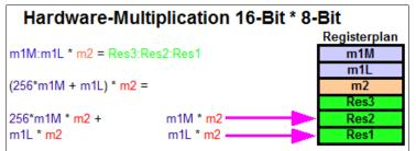
So the 16-bit-binary m1 is equal to 256\*m1M plus m1L, where m1M is the MSB and m1L is the LSB. Multiplying m1 by 8-bit-binary m2 so is, mathematically formulated:
