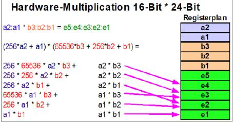
The multiplication of a 16 bit binary "a" with a 24 bit binary "b" leads to results with up to 40 bit length. The multiplication scheme requires six 8-by-8-bit multiplications and adding the results to the appropriate position in the result registers.
