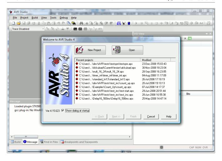
The first dialog asks whether an existing project should be opened or a new project is to be started. In case of a newly installed Studio "New Project" is the correct answer. The Button "Next>>" brings you to the settings dialog of your new project.
