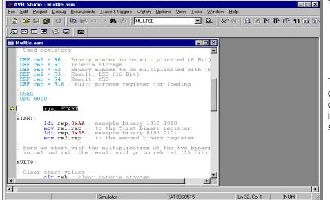
The object-code has been opened, the cursor is placed on the first executable instruction. F11 does single steps.
