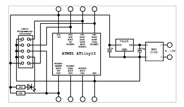
The ATtiny13 requires no external XTAL or clock generator, because it works with its internal 9.6 Mcs/s
