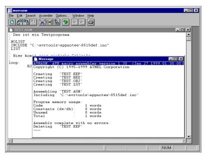
Klicking on the editor's external program caller or on the batch file starts the command line assembler. That piece of software reports the complete translation process (in the smaller window), here with no errors. If errors occur these are notified, along with their type and line number. Assembling resulted in one word of code which resulted from the RJMP instruction that we used. Assembling our single asm-text file now has produced four other files (not all apply here).
