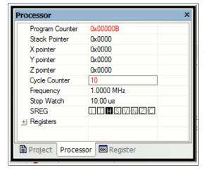
The cycle counter of the multiplication points to 10, at 1 MHz clock a total of 10 microseconds. Very much faster than software multiplication!
