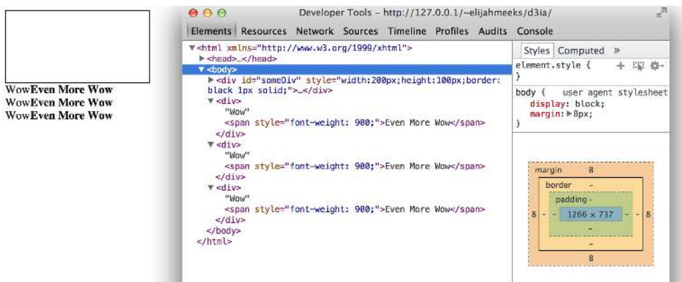
Figure 1.18 Inspecting the DOM shows that the new <div> elements have been created with unformatted content followed by the child <span> element with style and content set by your code.
