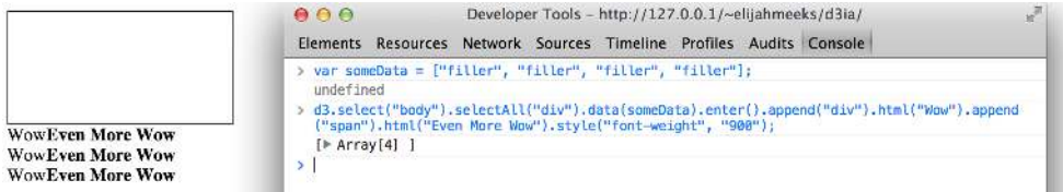
Figure 1.17 By binding an array of four values to a selection of <div> elements on the page, we can see that the .enter() function created three new <div> elements to reflect the size mismatch between the data array and the selection.
