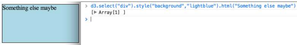
Figure 1.8 The D3 select syntax modifies style using the .style() function and traditional HTML content using the .html() function.
