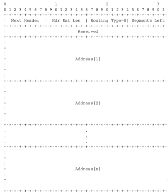
Fig. 3.54: The Type 0 routing header (RFC 2460)
