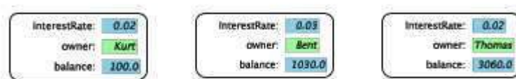
Figure 11.4 Three objects of class BankAccount , each holding three instance variables interestRate , owner , and balance . The values of variables are determined by the bank account transactions that we programmed in the class BankAccountClient . The state of the variables is shown relative to the three WriteLine calls.
