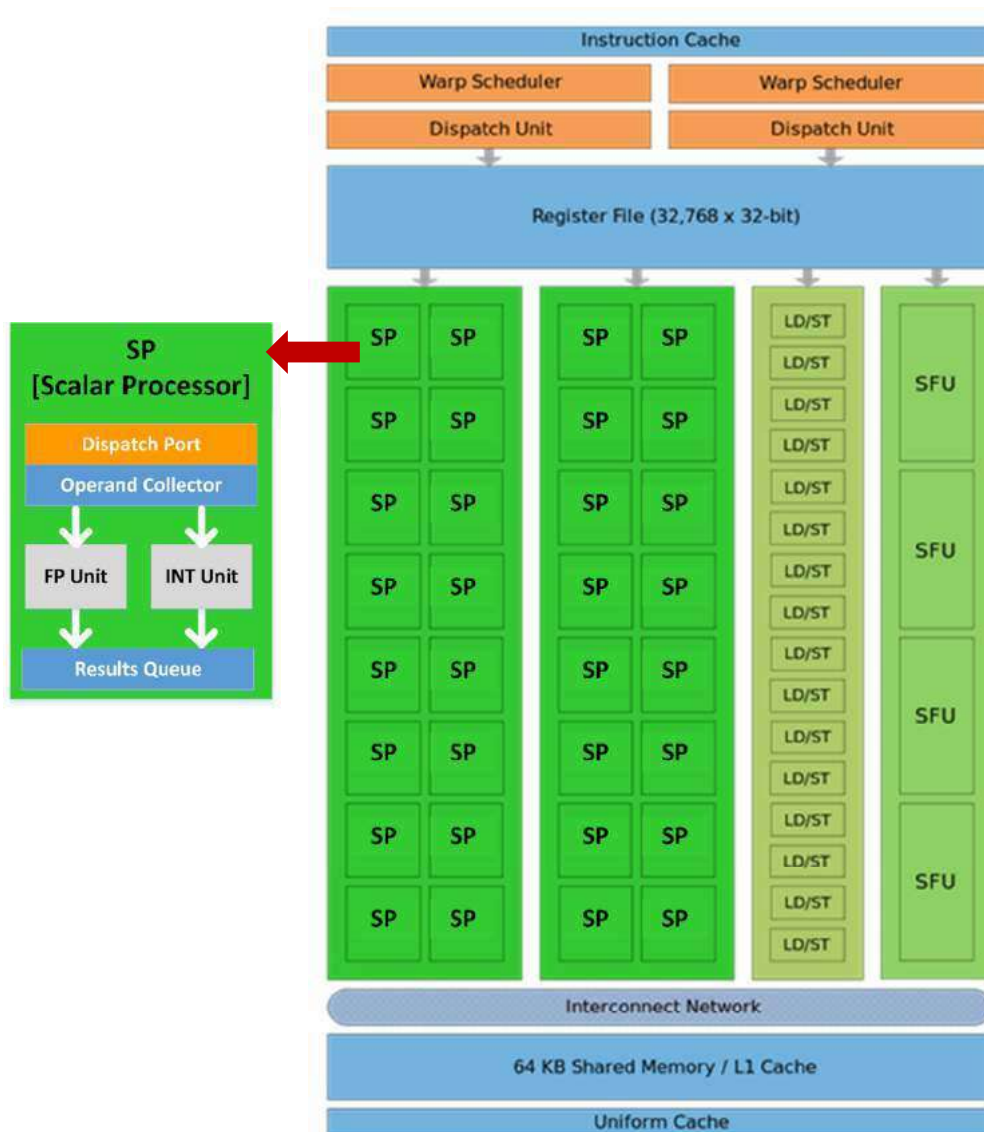
Figure 44. Architecture of a Stream Multiprocessor (SM). Fermi has four functional units: two blocks of 16 SPs each, a group of four SFUs, and a set of 16 load/store units. Color code: orange - scheduling and dispatch; green - execution; light blue - registers and caches. Credit: Nvidia.
