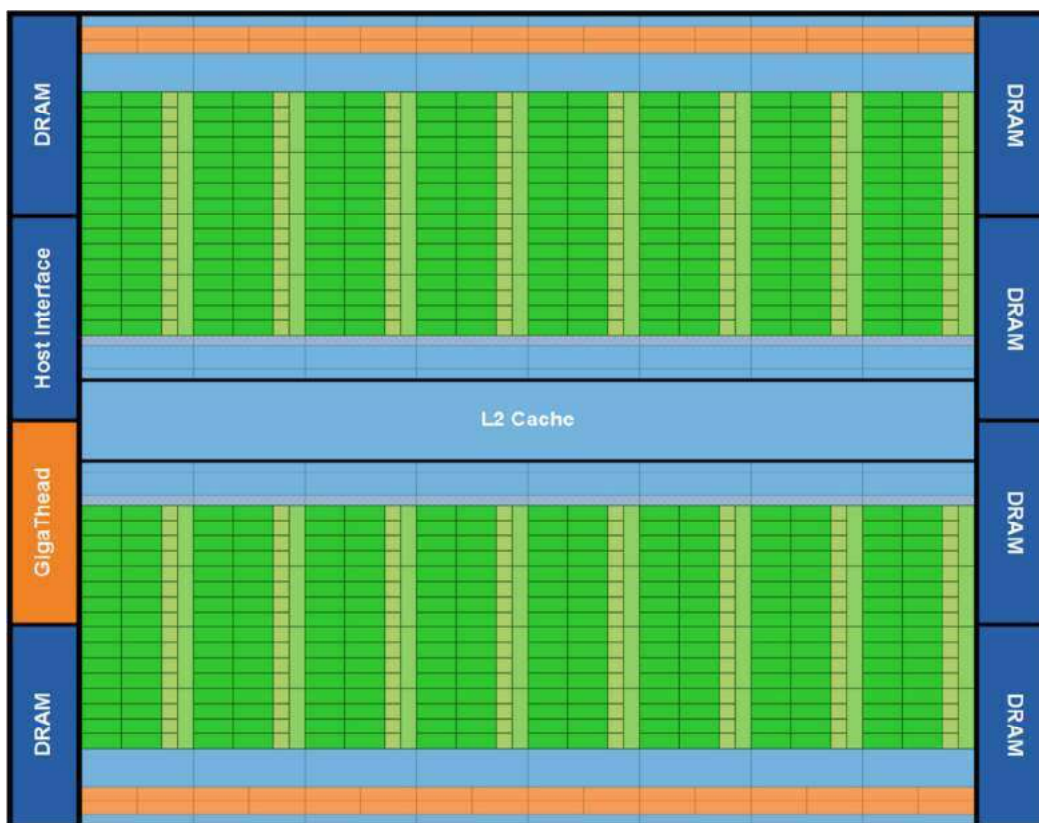
Figure 38. A schematic of the Fermi architecture. Color code: orange - scheduling and dispatch; green - execution; light blue – registers and caches. The co-processor is made up of a collection of 16 Stream Multiprocessors (SMs). Details of an SM are provided in Figure 44. Credit: Nvidia.
