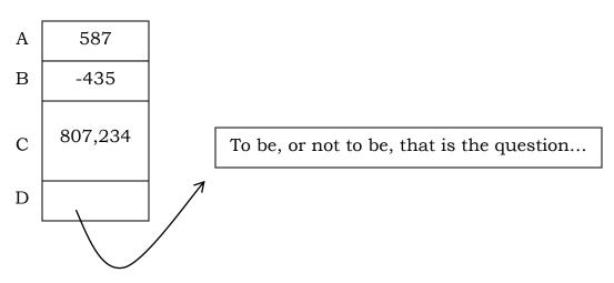
The string can be as small or as large as it needs to be, but the space on the stack required for the reference remains the same.
