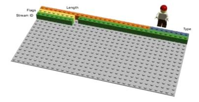
http2 sends binary frames. There are different frame types that can be sent and they all have the same setup: Length, Type, Flags, Stream Identifier, and frame payload.
