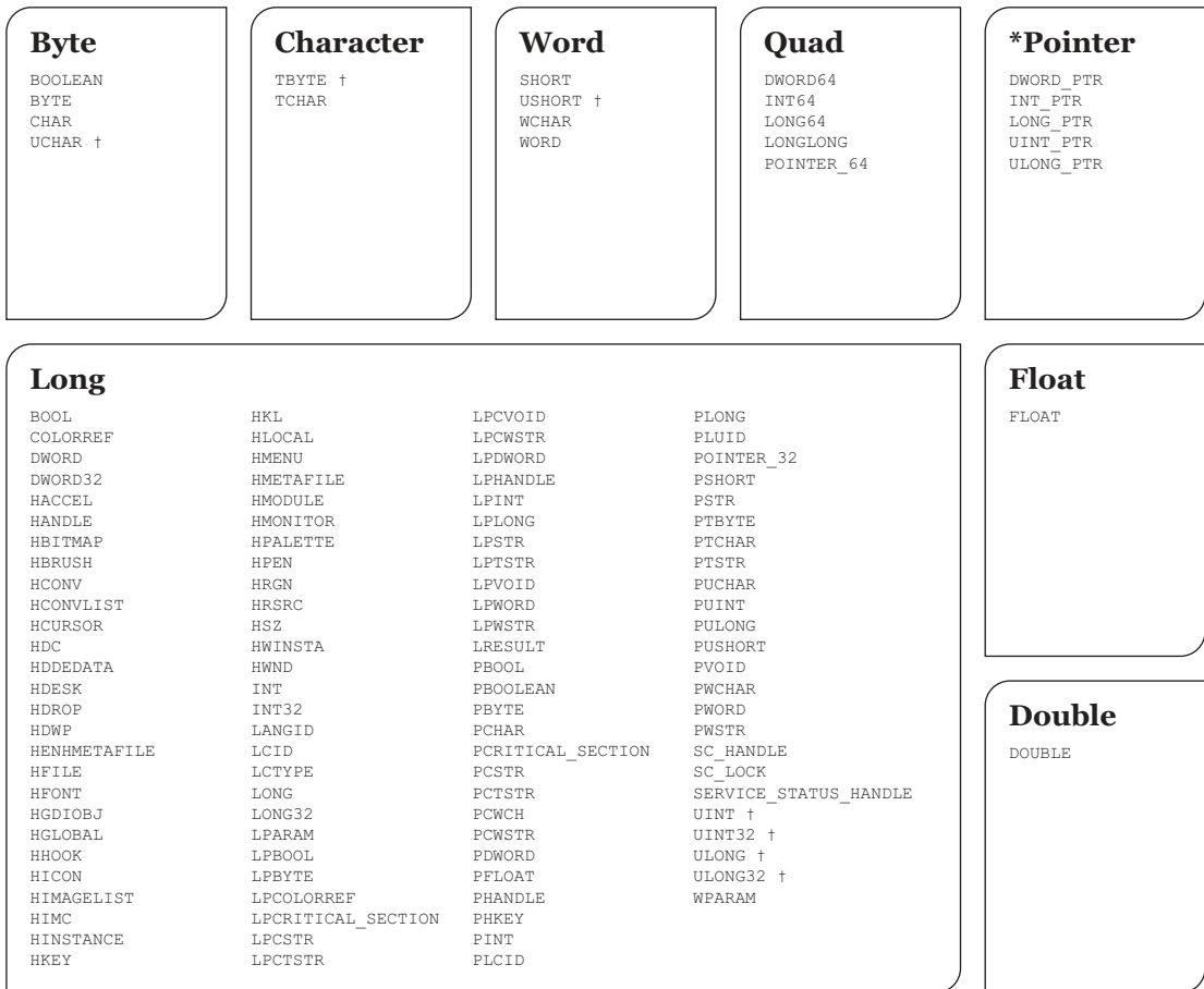
Types marked with ‘†’ need to be read correctly after a command call. This is because these types may be unsigned or signed opposite to the PureBasic type they are using.
