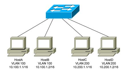
Four hosts are connected to a Layer-2 switch that supports VLANs:
