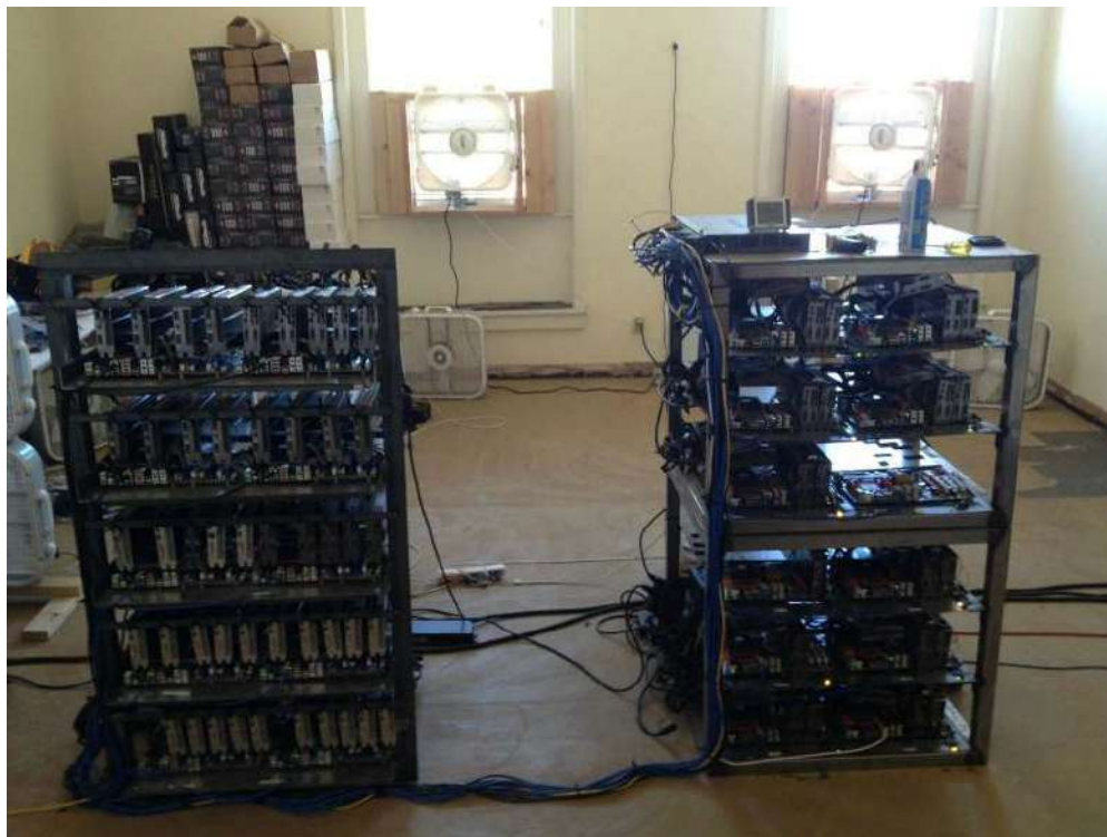
Figure 5.7: A home-built rack of GPUs used for Bitcoin mining. You can also see the fans that they used to build a primitive cooling system. Source: LeonardH, cryptocurrenciestalk.com.
