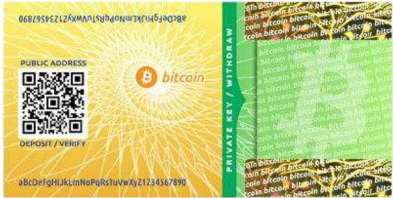
Figure 4.3: A Bitcoin paper wallet with the public key encoded both as a 2D barcode and in base 58 notation. Observe that the private key is behind a tamper-evident seal.
