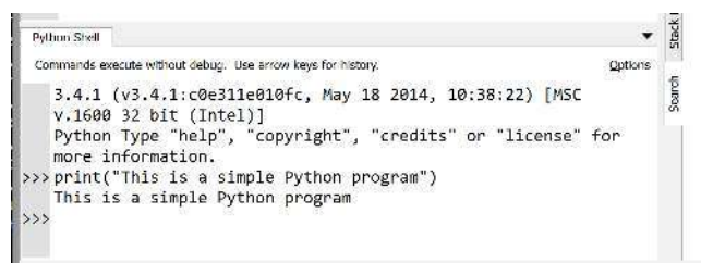
Figure 1.13 The interactive shell allows us to submit Python statements and expressions directly to the interpreter
