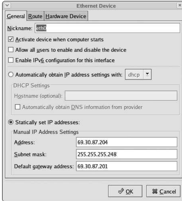
Figure 2-4 The Ethernet Device window in the Fedora Core Network Configuration Tool
