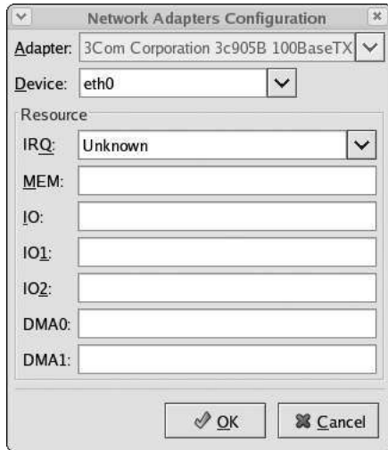
Figure 2-6 The Network Adapters Configuration window
