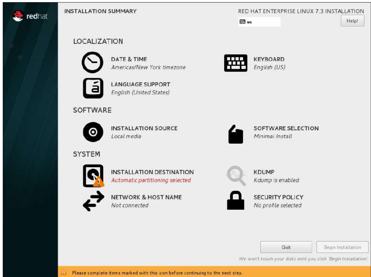
Figure 2.1. The Installation Summary screen
